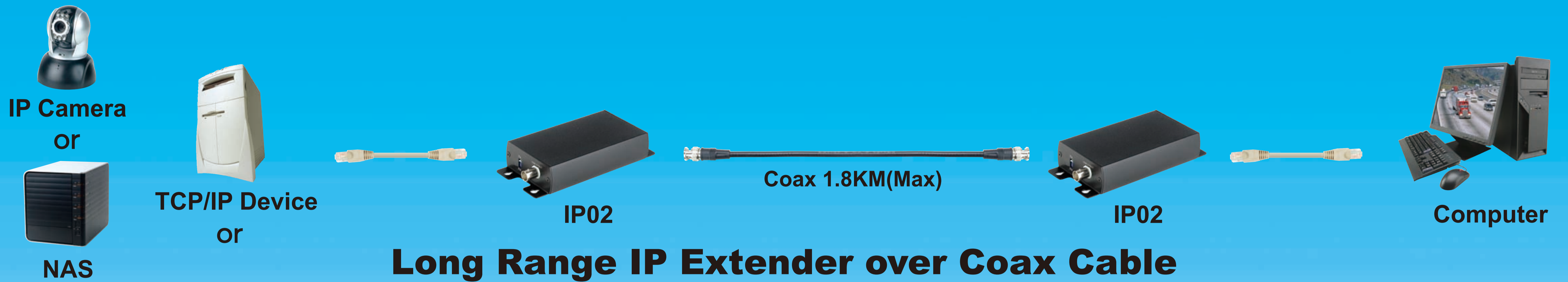
4 IP Cameras over Coax Cabling Solution
