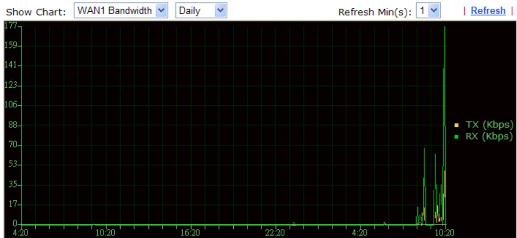
The horizontal axis represents time. Yet the vertical axis has different meanings. For WAN1 Bandwidth chart, the numbers displayed on vertical axis represent the numbers of the transmitted and received packets in the past.
