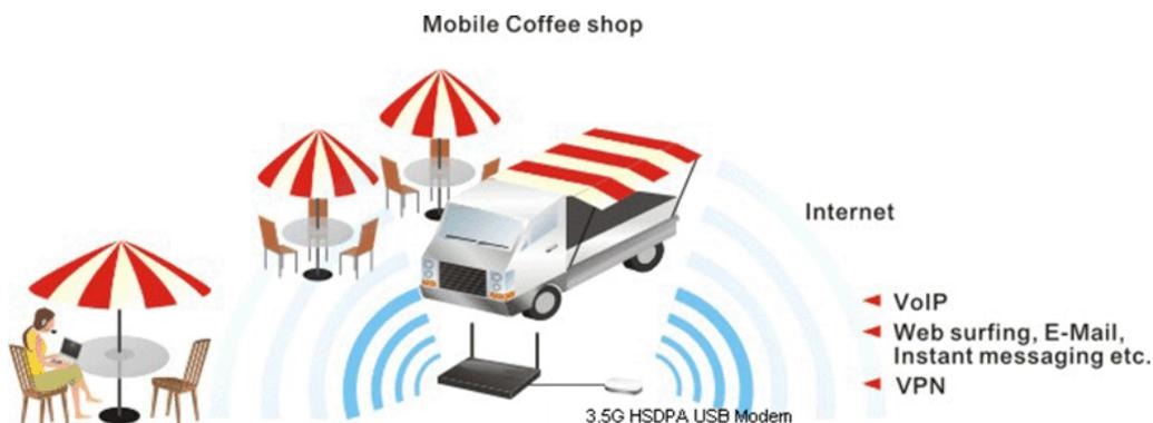
After connecting into the router, 3G USB Modem will be regarded as the backup WAN port. Therefore, when WAN is not available, the router will use 3.5G for supporting automatically. The supported 3G USB Modem will be listed on DrayTek web site. Please visit [www.draytek.com](http://www.draytek.com) for more detailed information.
