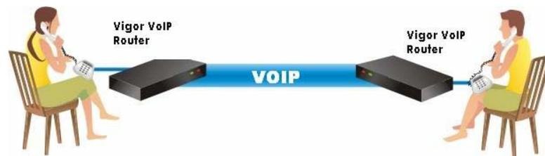
Our Vigor V models firstly apply efficient codecs designed to make the best use of available bandwidth, but Vigor V models also equip with automatic QoS assurance. QoS Assurance assists to assign high priority to voice traffic via Internet. You will always have the required inbound and outbound bandwidth that is prioritized exclusively for Voice traffic over Internet but you just get your data a little slower and it is tolerable for data traffic.
