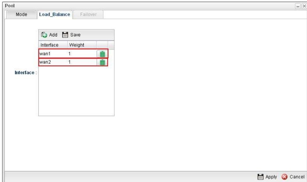
Setup the Weights (e.g, "1") of WAN1 and WAN2 as you want. In this case ratio of WAN1 and WAN2 is 1:1. Also, you can type 2 and 1 for WAN1 and WAN2, then the ratio of line speed of WAN 1 and line speed of WAN 2 will be 2:1.
