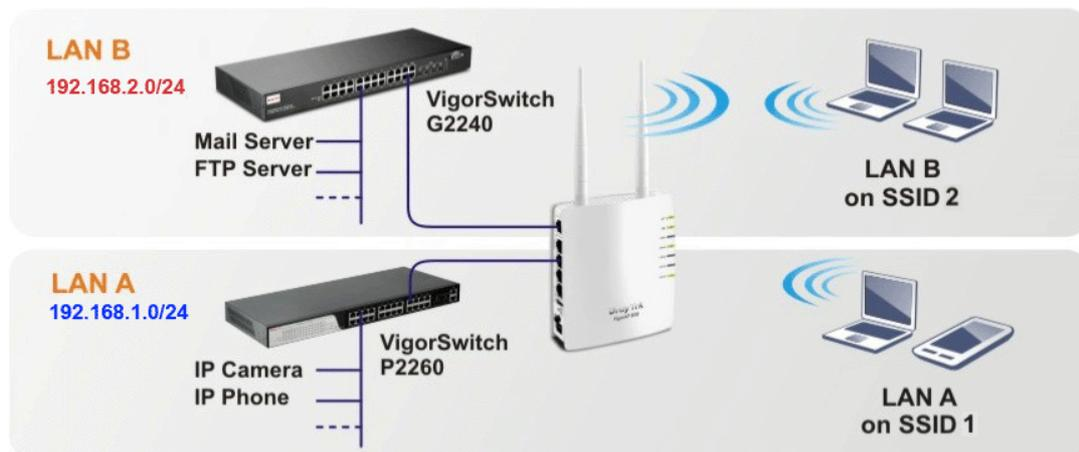
In the above figure, VigorAP 800 is used to control the wireless network connection. It can separate the wireless traffic between accessing internal server and the usage of video. Wireless station connecting to VigorAP 800 with SSID 1 can get the IP address with the network segment of 192.168.1.0/24 (LAN-A); wireless station connecting to VigorAP800 with SSID 2 can get the IP address with the same network segment of 192.168.2.0/24 (LAN-B).
