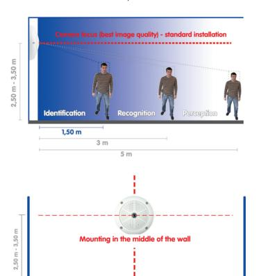
Recommendation: Mounting the camera in the middle of the wall
