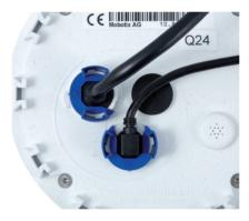
Open the cable retainer by rotating the bayonet catch to the marked position
