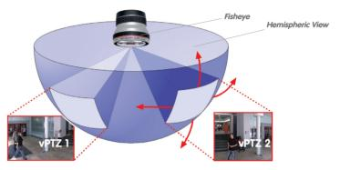
When ceiling mounted, the image area of the hemispheric camera covers the entire room. The image in the hemisphere is convex, particularly near the image borders. These image sections are corrected for the viewer by the integrated distortion correction software, allowing a view of the scene from the usual perspective. The **virtual PTZ feature** allows you to enlarge or move image sections within the hemisphere, just like a PTZ camera yet, with MOBOTIX, this is achieved with no moving parts.
