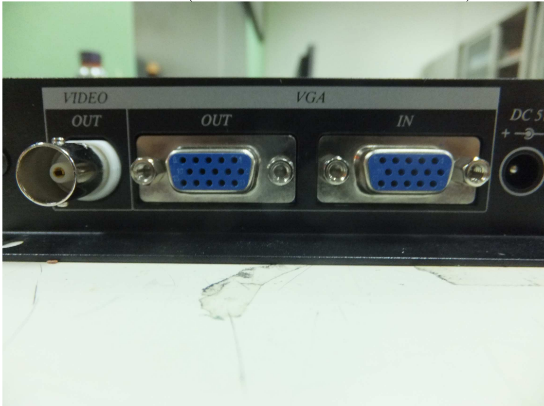
03 IO Port of EUT(Video out & VGA IN &VGA OUT & DC IN )
