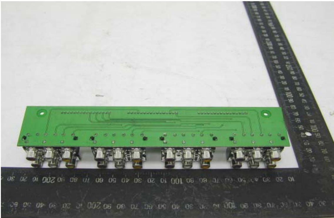
Solder Side of Main Board 2
