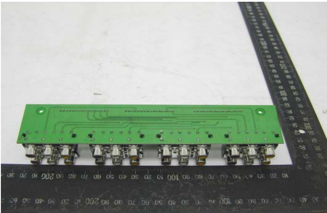
Solder Side of Main Board 2
