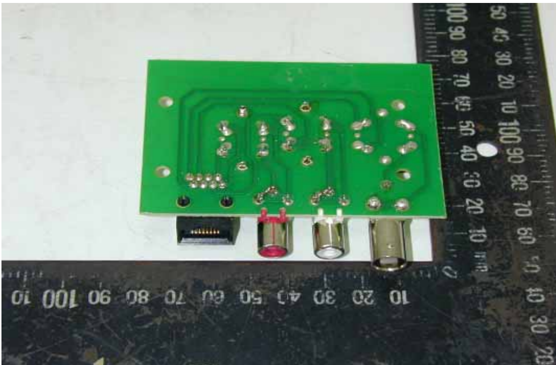
Solder Side of Main Board
