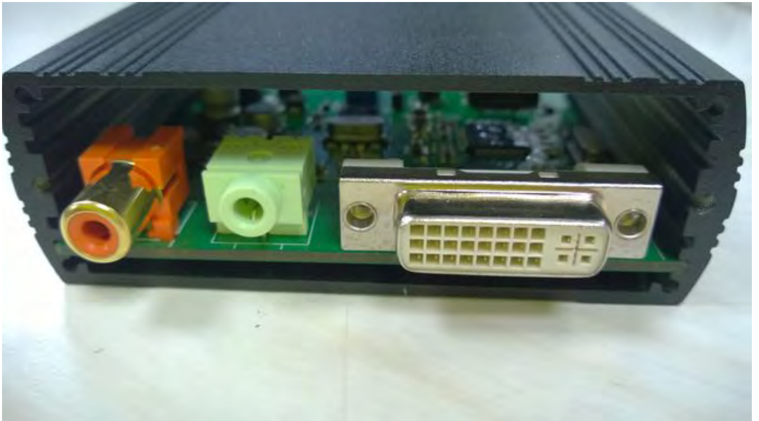
06 Inside Port of EUT (DVI & RCA & 3.5mm Phone Jack)
