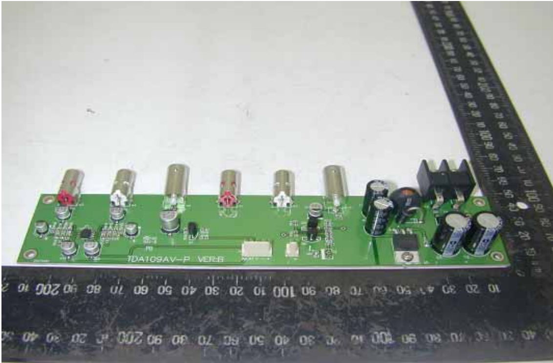
Component Side of Main Board 2
