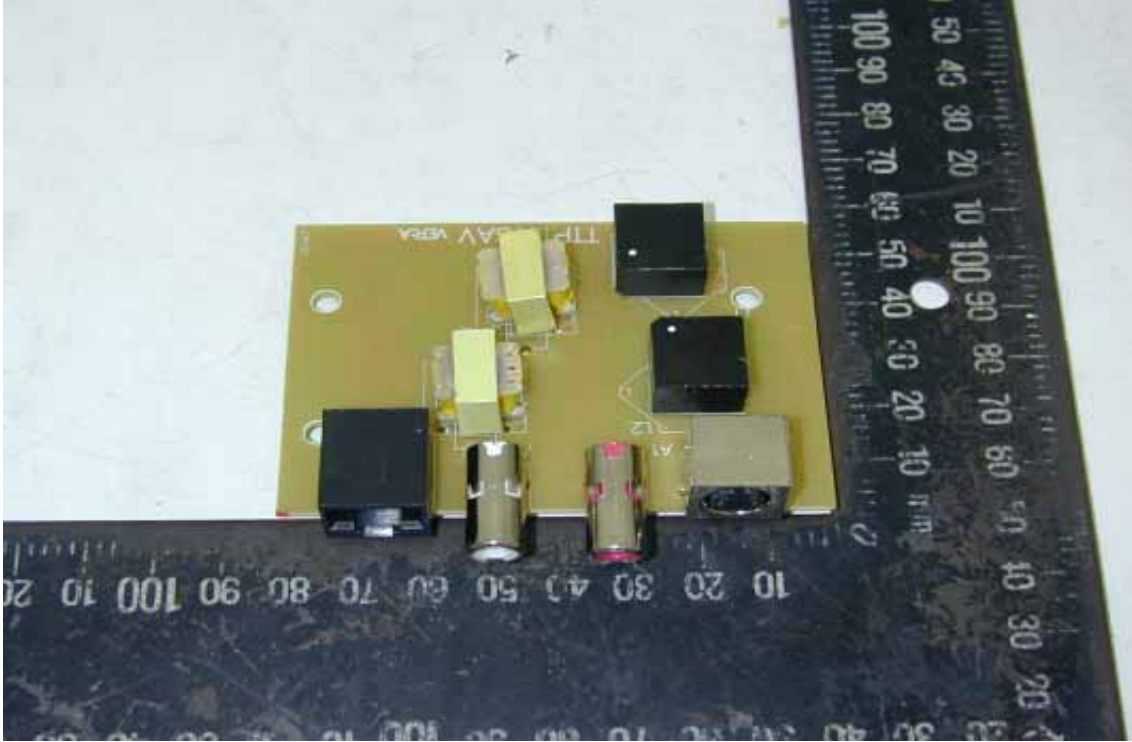
Component Side of Main Board
