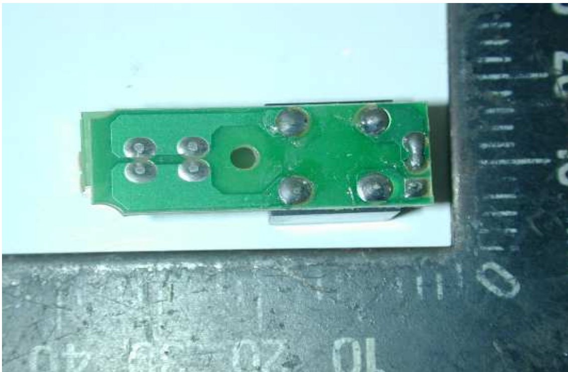
Solder Side of Main Board
