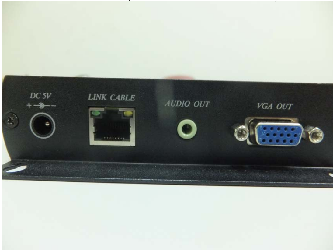
03 IO Port of EUT(DC IN & RJ45 & Audio OUT & VGA)
