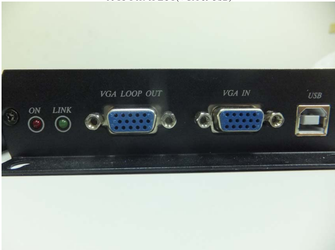
06 IO Port of EUT(VGA & USB)
