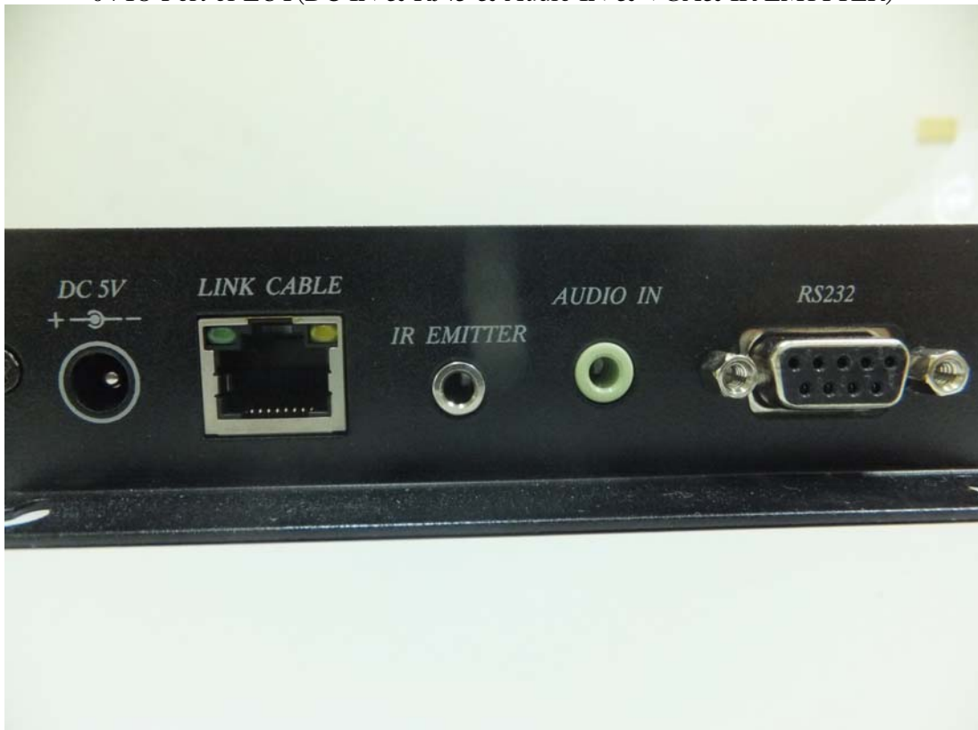
04 IO Port of EUT(DC IN & RJ45 & Audio IN & VGA & IR EMITTER)
