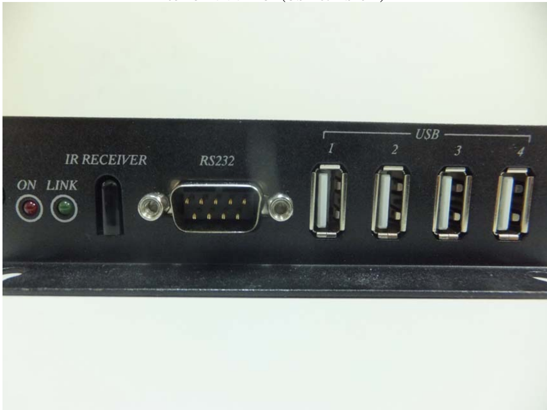
05 IO Port of EUT(USB & RS232 )
