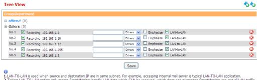
1.LAN-TO-LAN is used when source and destination IP are in same subnet. For example, accessing internal mail server is typical LAN-TO-LAN application.
