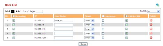
1.LAN-TO-LAN is used when source and destination IP are in same subnet. For example, accessing internal mail server is typical LAN-TO-LAN application.
