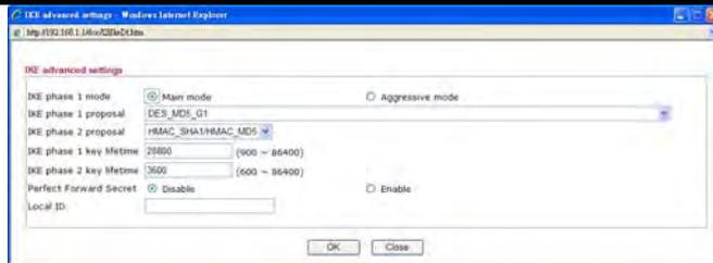
**IKE phase 1 mode** -Select from **Main** mode and **Aggressive** mode. The ultimate outcome is to exchange security proposals to create a protected secure channel. **Main** mode is more secure than **Aggressive** mode since more exchanges are done in a secure channel to set up the IPSec session. However, the **Aggressive** mode is faster. The default value in Vigor router is Main mode.
