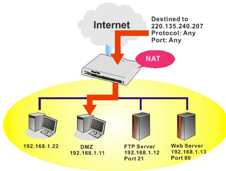
The security properties of NAT are somewhat bypassed if you set up DMZ host. We suggest you to add additional filter rules or a secondary firewall.
