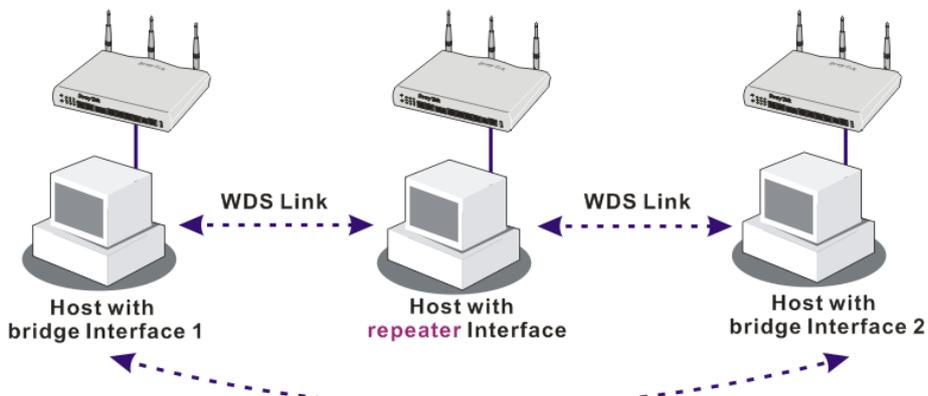
The major difference between these two modes is that: while in **Repeater** mode, the packets received from one peer AP can be repeated to another peer AP through WDS links. Yet in **Bridge** mode, packets received from a WDS link will only be forwarded to local wired or wireless hosts. In other words, only Repeater mode can do WDS-to-WDS packet forwarding.
