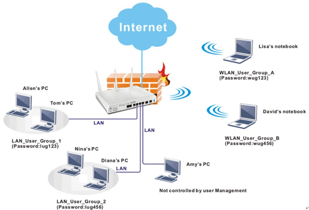
**Note:** Filter rules configured under Firewall usually are applied to the host (the one that the router installed) only. With user management, the rules can be applied to every user connected to the router with customized profiles.
