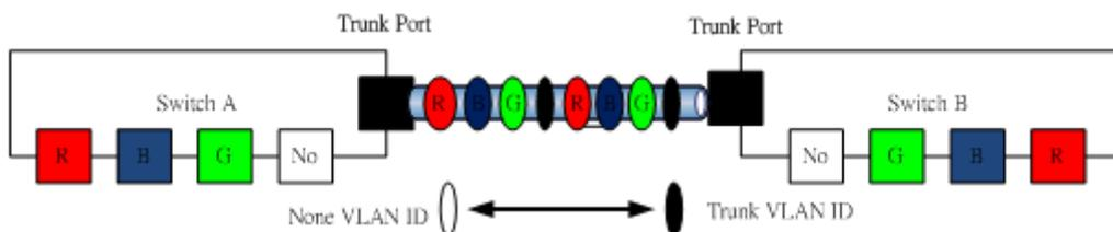
Trunk Port can carry the packets with VID but replace the Non-VID packet as the VID of Trunk port while forwarding the packets to another switch.
