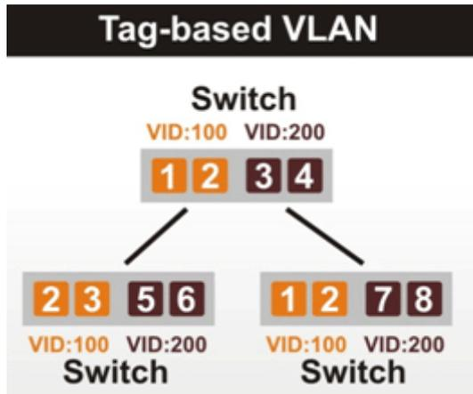
Vigor routers <sup>[Note]</sup> support Tag-based feature both on LAN and WAN interfaces. The next we'll demonstrate our web design and how to configure the settings by introducing the functionalities of Vigor router.
