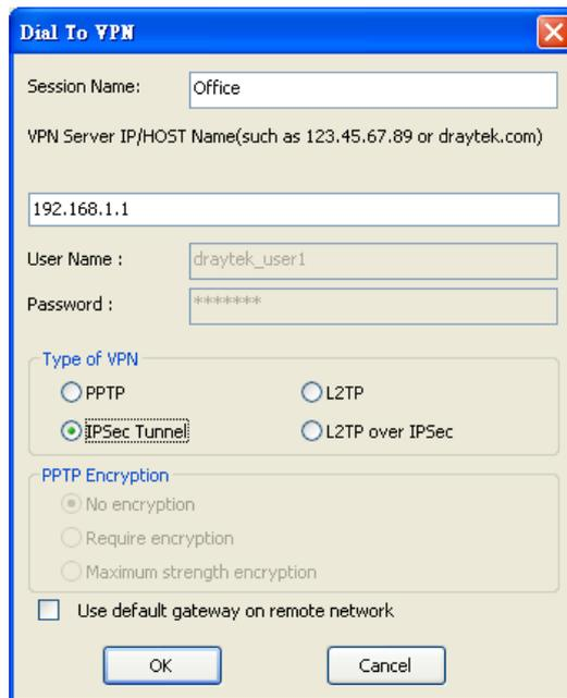
You may further specify the method you use to get IP, the security method, and authentication method. If the Pre-Shared Key is selected, it should be consistent with the one set in VPN router.
