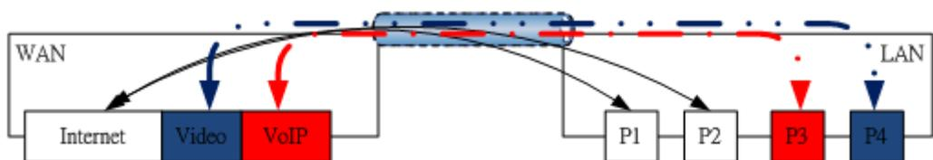
P1 and P2 are doing NAT flow to access to the internet, but P3 and P4 will forward the packets between WAN and LAN ports directly.
