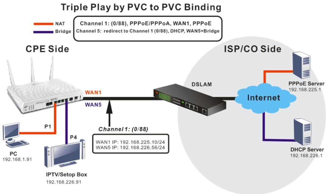
From the above figure, Setop Box and DHCP server can reach for each other through WAN5 with Bridge mode; LAN PC in P1 beneath Vigor router can reach to PPPoE Server through WAN1 with NAT. Both NAT and Bridge are built through the same Channel 1.
