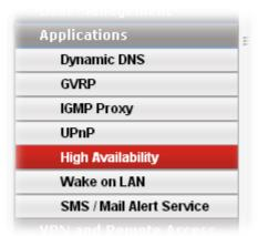
3. In the tab of **High Availability Global Setup**, choose **Hot-Standby** as Redundant Method; choose **Primary** as Config Synchronization Rule; type **draytek** as Authentication Key; choose **Immediate** as Advance Preemption Mode. Click **Apply** to save the settings.
