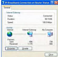
The UPnP facility on the router enables UPnP aware applications such as MSN Messenger to discover what are behind a NAT router. The application will also learn the external IP address and configure port mappings on the router. Subsequently, such a facility forwards packets from the external ports of the router to the internal ports used by the application.
