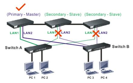
When the Master device fails, one of the slave devices will be chosen as the Master device to offer the network service for the connected PCs.
