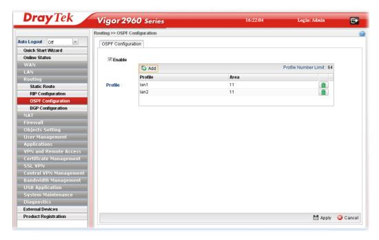
5. After setting, check the routing information (marked with red line) which is created by OSPF
