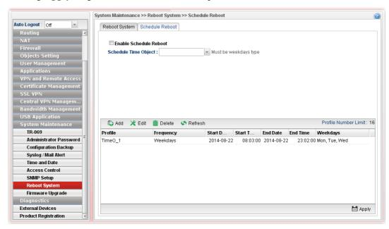
Usually, you have to configure required time object from **Objects Setting>>Time Object** before choosing it for applying. If you do not create any time object previously, you can also create a required one in this page directly. The bottom of this page offers tools for you to create time object. The way of configuration is the same as settings in **Objects Setting>>Time Object**.
