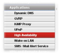
3. In the tab of **High Availability Global Setup**, choose **Hot-Standby** as Redundant Method; choose **Secondary** as Config Synchronization Rule; type the lan1 IP address configured in router A; type **draytek** as Authentication Key; choose **Automatic** as Advance Preemption Mode. Click **Apply** to save the settings.
