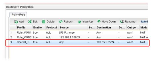
Now, any packets from LAN1 sent to the remote PC (IP address: 203.65.1.35) will be forcefully to pass through WAN1.
