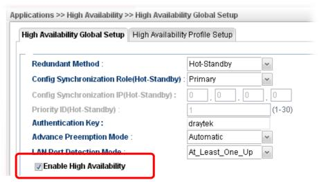
Under such construction, when Router A (defined as Master device) is powered off, Router B (defined as Slave device) will be up and take over all the jobs that Router A performs. Later, when Router A is powered on again, all the jobs will return to Router A.
