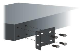
After the bracket installation, the Vigor3900 Series chassis can be installed in a rack by using four screws for each side of the rack.
