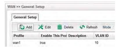
5. Create a new WAN profile named with **wan1\_1**, and set VLAN ID named with **111** based on WAN Port 1(WAN1). Note that **Untag** must be set with **Disable**. It means wan1\_1 can accept the packets tagged with VLAN ID 111. Next, click **Apply** to save the settings.
