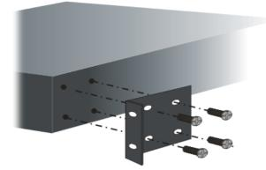
After the bracket installation, the Vigor3912 Series chassis can be installed in a rack by using four screws for each side of the rack.
