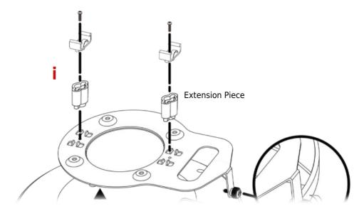
vi. Attach the T-Rail brackets to the ceiling frame.
