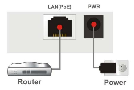
• Connect VigorAP to the PoE switch (via LAN port) with an Ethernet cable for getting the power from the switch directly. While connecting with a PoE switch, the power adapter is not necessary but optional.
