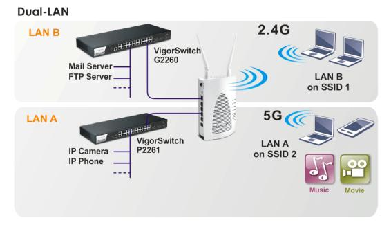
In the above figure, VigorAP 900 is used to control the wireless network connection. It can separate the wireless traffic between accessing internal server and the usage of video. Wireless station connecting to VigorAP 900 with SSID 2 can get the IP address with the network segment of 192.168.1.0/24 (LAN-A); wireless station connecting to VigorAP 900 with SSID 1 can get the IP address with the same network segment of 192.168.2.0/24 (LAN-B).
