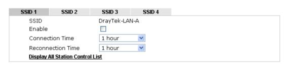
Note: Once the feature is enabled, the connection time quota will apply to each wireless client (identified by MAC address).
