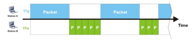
It is similar to automatic Bandwidth Limit. The dynamic bandwidth limit of each station depends on instant active station number and airtime assignment. Please note that Airtime Fairness of 2.4GHz and 5GHz are independent. But stations of different SSIDs function together, because they all use the same wireless channel. IN SPECIFIC ENVIRONMENTS, this function can reduce the bad influence of slow wireless devices and improve the overall wireless performance.
