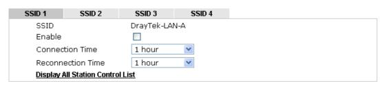
Note: Once the feature is enabled, the connection time quota will apply to each wireless client (identified by MAC address).
