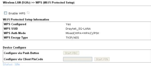
Note: WPS can help your wireless client automatically connect to the Access point.
