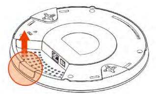
• Connect VigorAP to Vigor router (via LAN port) with Ethernet cable.
