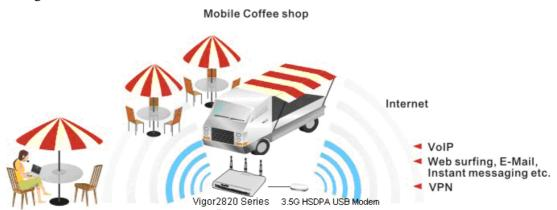
After connecting into the router, 3G USB Modem will be regarded as the second WAN port. However, the original Ethernet WAN1 still can be used and Load-Balance can be done in the router. Besides, 3G USB Modem in WAN2 also can be used as backup device. Therefore, when WAN1 is not available, the router will use 3.5G for supporting automatically. The supported 3G USB Modem will be listed on Draytek web site. Please visit www.draytek.com for more detailed information.
