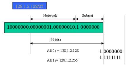
In this diagram, you can see the subnet mask with 25-bit long, 255.255.255.128, contains 126 members in the sub-netted network. Another is that the length of network prefix equals the number of the bit with 1s in that subnet mask. With this, you can easily count the number of IP addresses matched. The following table shows the result.
