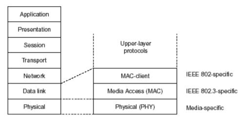
In the above figure, we can see that Ethernet locates at the Data Link layer and Physical layer and comprises three portions, including logical link control (LLC), media access control (MAC), and physical layer. The first two comprises Data link layer, which performs splitting data into frame for transmitting, receiving acknowledge frame, error checking and re-transmitting when not received correctly as well as provides an error-free channel upward to network layer.
